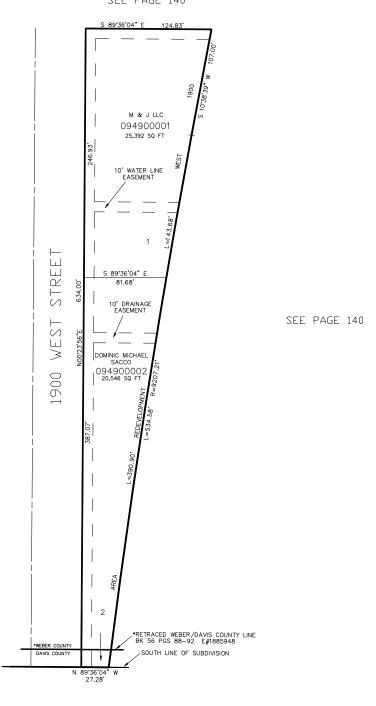
10' UTILITY & DRAINAGE EASEMENTS EACH SIDE OF PROPERTY LINES AS INDICATED BY DASHED LINES EXCEPT AS OTHERWISE SHOWN.
